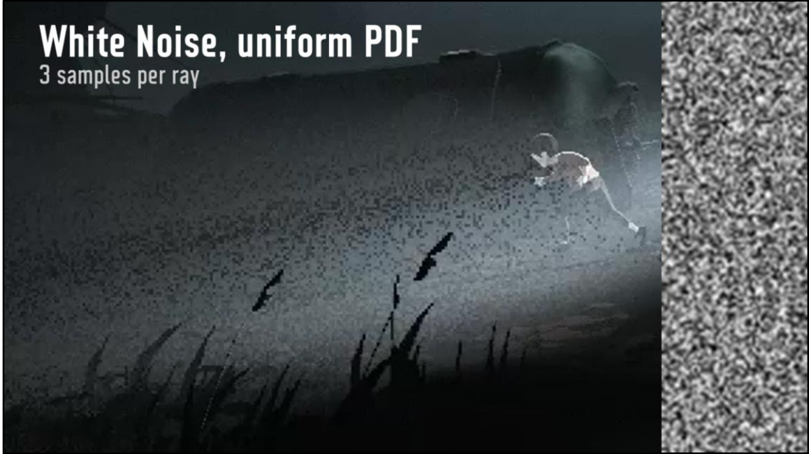
same image as before, but with 3 samples instead of 32... shadow effect barely recognizable massive undersampling, loads of noise
